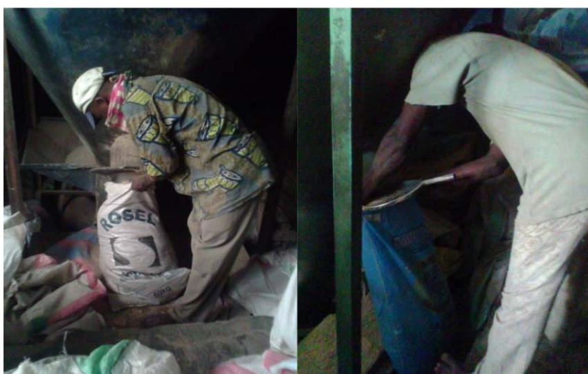
Figure 5. Discharge operation; filling bags with feed (left), opening discharge gate (right).
