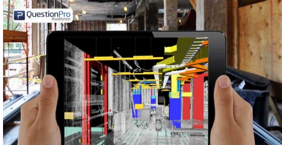
Figure 2. Augmented Reality in Construction Used on an iPad [9]
