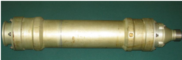
Fig.3. General view of the submersible asynchronous motor MASUM-10
