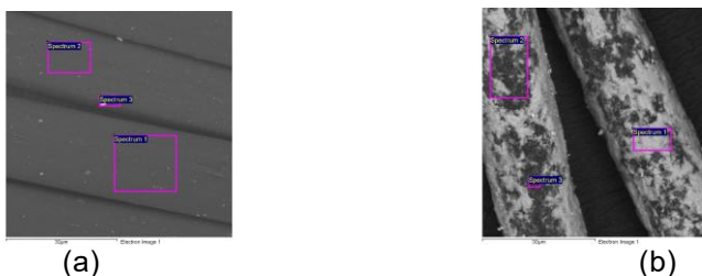
Figure 4: EDX images of (a) untreated and (b) treated polyamide samples
