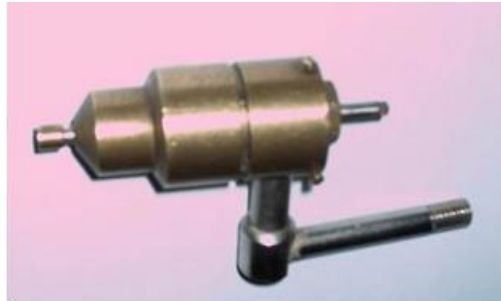
Fig. 1. Experimental air-jet ultrasonic generator
