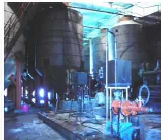
Fig. 5. Hydroacoustic cavitation installation in the department for clarification and stabilization of wines (Stauceni winery)
