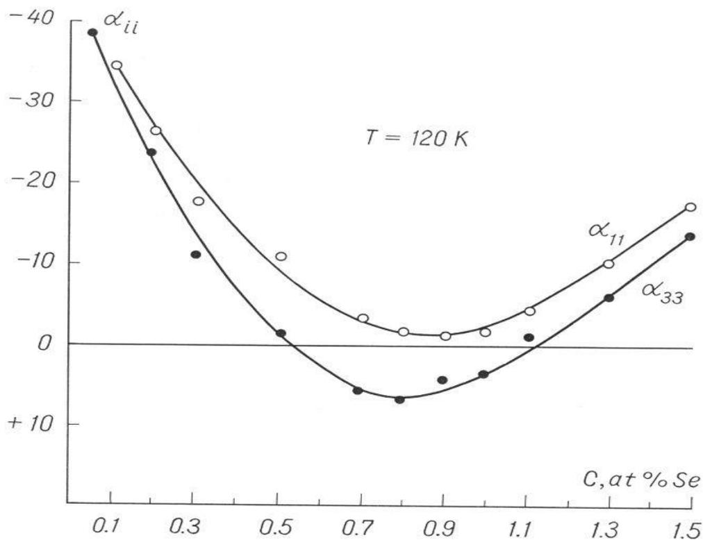
Fig. 2 Concentration dependence of the thermopower  $\alpha_{ii}(c)$  at the temperature  $T=120$  K.
