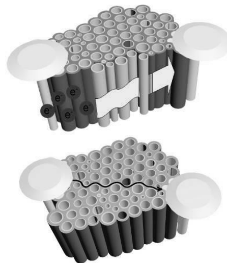
Fig 2. Carrier density of nanoporous InP is represented by grey color and with solid arrow/line show a conductive pathway.
