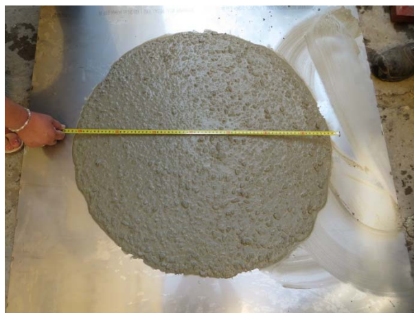
Figure 1. Slump flow test of SCC.
