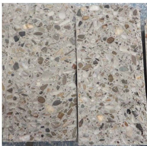
Figure 3. Structure of SCC.
