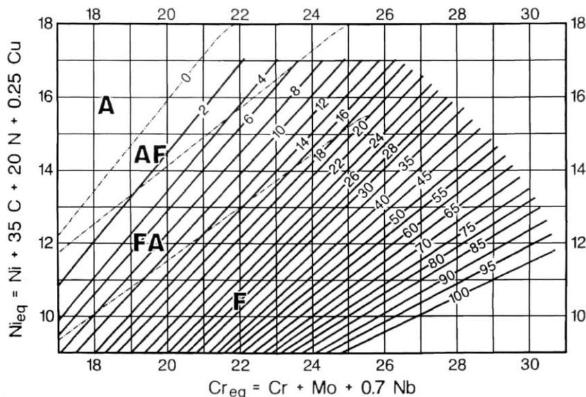
Figure 1. The WRC-1992 reference diagram Koteki & Siewert
