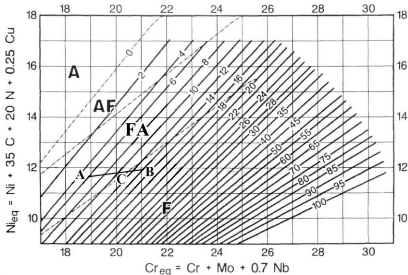
**Figure 3.** The determination of the ferrite content at the welded steel 10TiMoNiCr175 with stain 19.12.2 Nb electrodes
