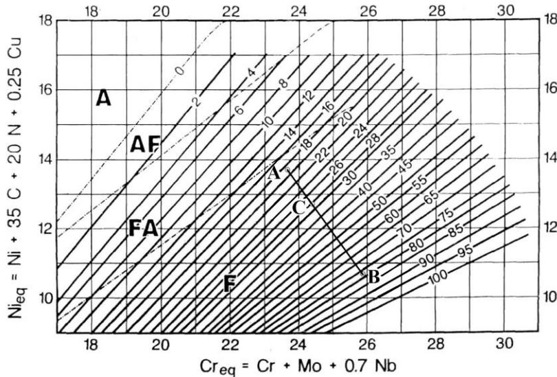
**Figure 2.** The determination of the ferrite content at the basis metal MB welding with the additional metal MA
