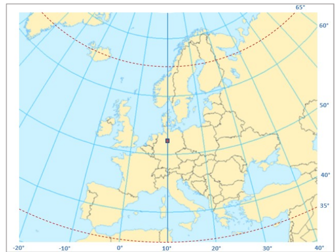
Figure 9. The Europe in Lambert Conformal Conic Projection
