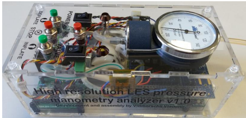
Fig. 4. “High Resolution LES Pressure Manometry Analyzer” test bench test.
