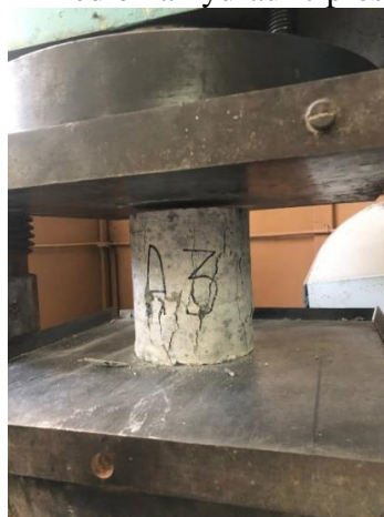
Figure 8. Testing a core of a reinforced concrete road slab on a press
