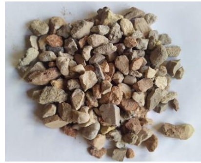
Figure 14. Secondary crushed stone from masonry and ceramic tiles (fractions of 8-16 mm)
