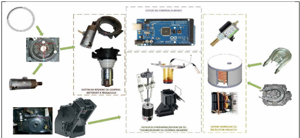
Fig. 9. Structural diagram of the electromechanical system of the innovative coffee machine with inductive heater [developed by the author]
