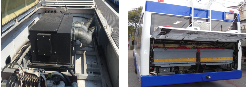
Figure 6. The traction and battery supply system for electric buses
