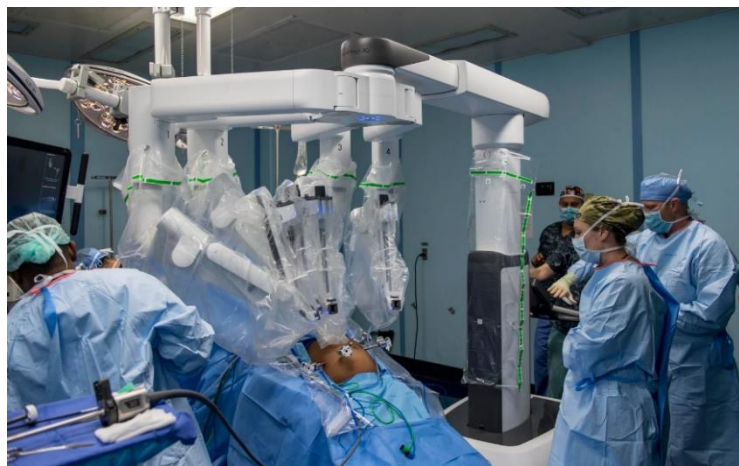
Figure 4. The da Vinci surgical robot. Photo taken on a US Navy hospital ship [10]
