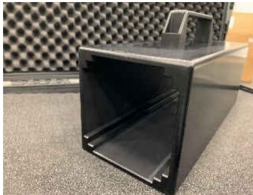
Figure 4.5. The model for confirming the fit of the satellite with the JSSOD launcher.
