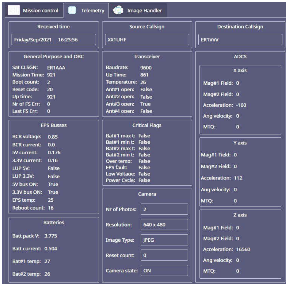
Figure 5.11. Example of information representation of a beacon message received from the TUMnanoSAT nanosatellite.
