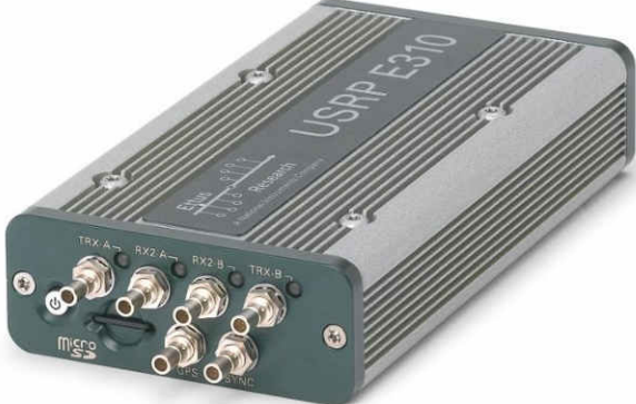
Figure 5.3. USRP E310 hardware device for SDR architecture.
