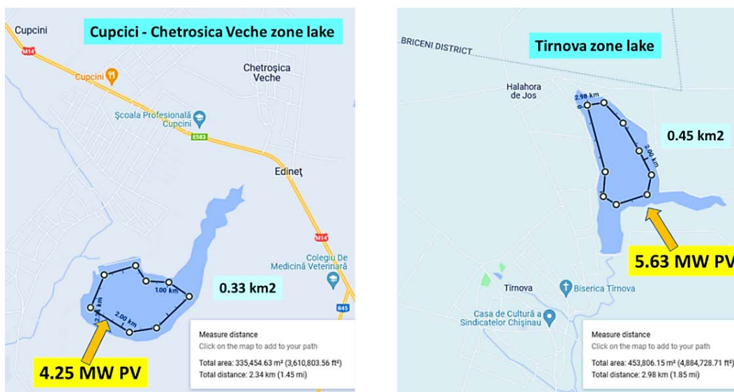
Figure 10. The potential of photovoltaic capacity for two small lakes and a potential formation of energy communities.
