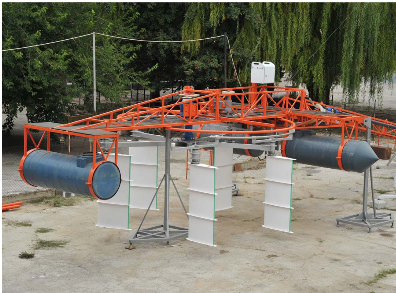
Figure 5. Industrial prototype of the micro-hydro power plant with modified hydrodynamic rotor for water kinetic energy conversion into electrical and mechanical energy.
