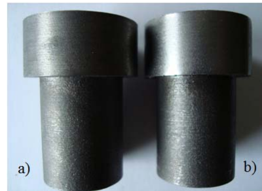
Figure 4. Work pieces: a) turning and b) the workpiece after cold plastic deformation by roller with ball bearing.
