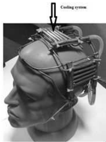
Fig. 1 The location of Peltier elements and cooling system on the human head
