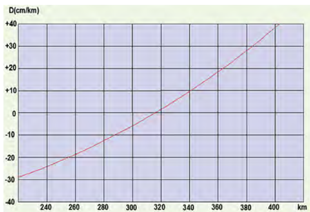
Fig. 6. Diagram of relative linear deformations for Stereo 70 map projection
