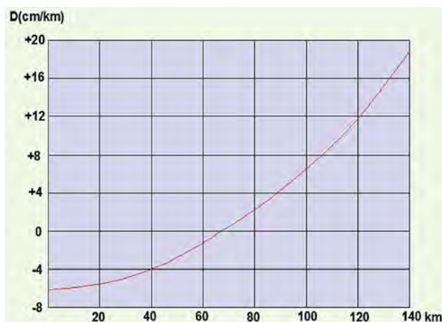
Fig. 4. Diagram of relative linear deformations for Transversal Mercator map projection
