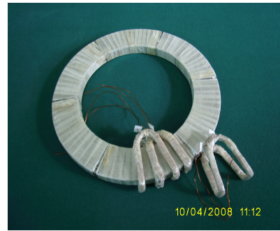
Fig. 2 Axial synchronous generators with permanent magnets with stator package without notches.
