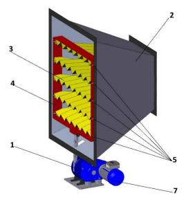
**Conclusions.** 1. Uniform distribution of air in the cross section of the drying chamber was ensured; 2. It was ensured the adjustment of the uniformity of the distribution according to the speed of the air passing between the profiled panels using their oscillating movement.
