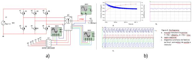
**Figure 5.** Actuation system with brushless DC motor: a) Multisim scheme; b) Extracted diagrams.
