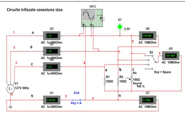
**Figure 2.** Multisim assembly for the study of three-phase electrical circuits, star connection.
