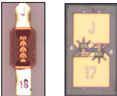
Fig. 2. Representative structures of diamond-based varactor (left) and film varistor (right) Schottky diodes developed by ACST.
