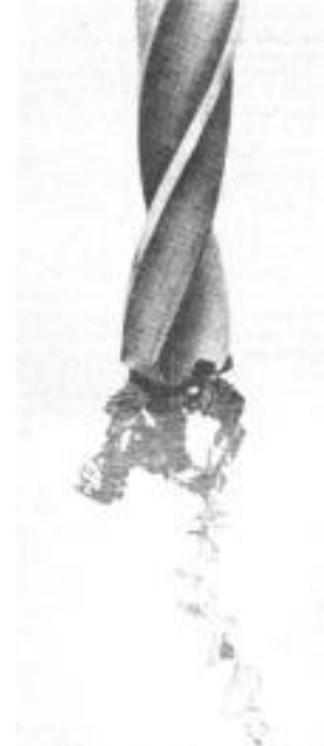
Figure 1. Magnetized drill shavings from a nonmagnetic titanium alloy VT1 - 0, holding it by the magnetic fluid.
