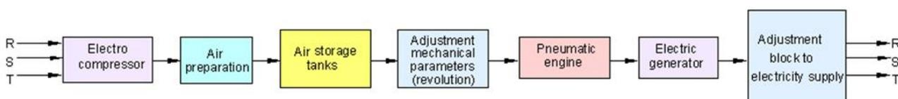
Fig. 16. Block diagram of a system for the capture, conversion and storage, in pneumatic energy
