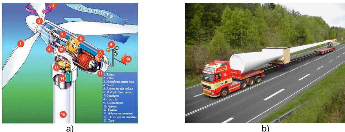
Fig. 11. The components of a wind energy conversion system (a) and turbine blade length of 62 m (b)
