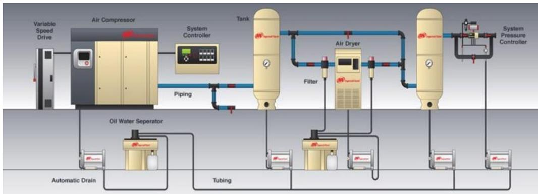
Fig. 19. Compressed air plant diagram (photo: creditkpowersystems.com) [16],
