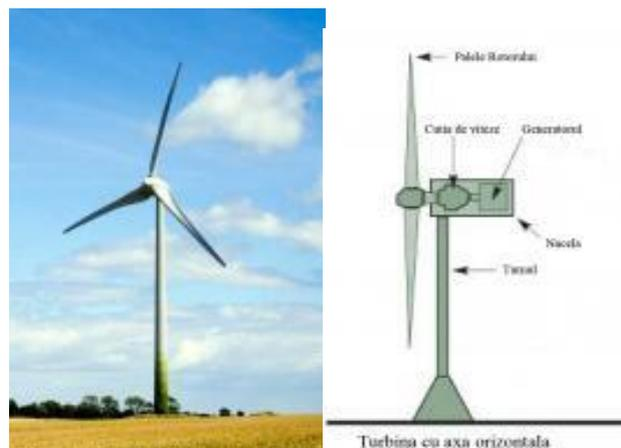
Fig. 10. Horizontally axis turbine [5]
