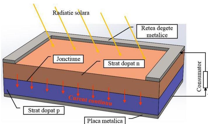
Fig. 6. Structure and functioning of photovoltaic cell [5]
