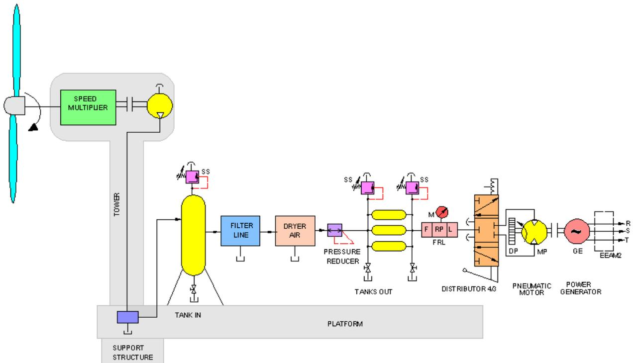
**Fig. 18.** Wind energy capture system, direct conversion and storage of the pneumatic energy
