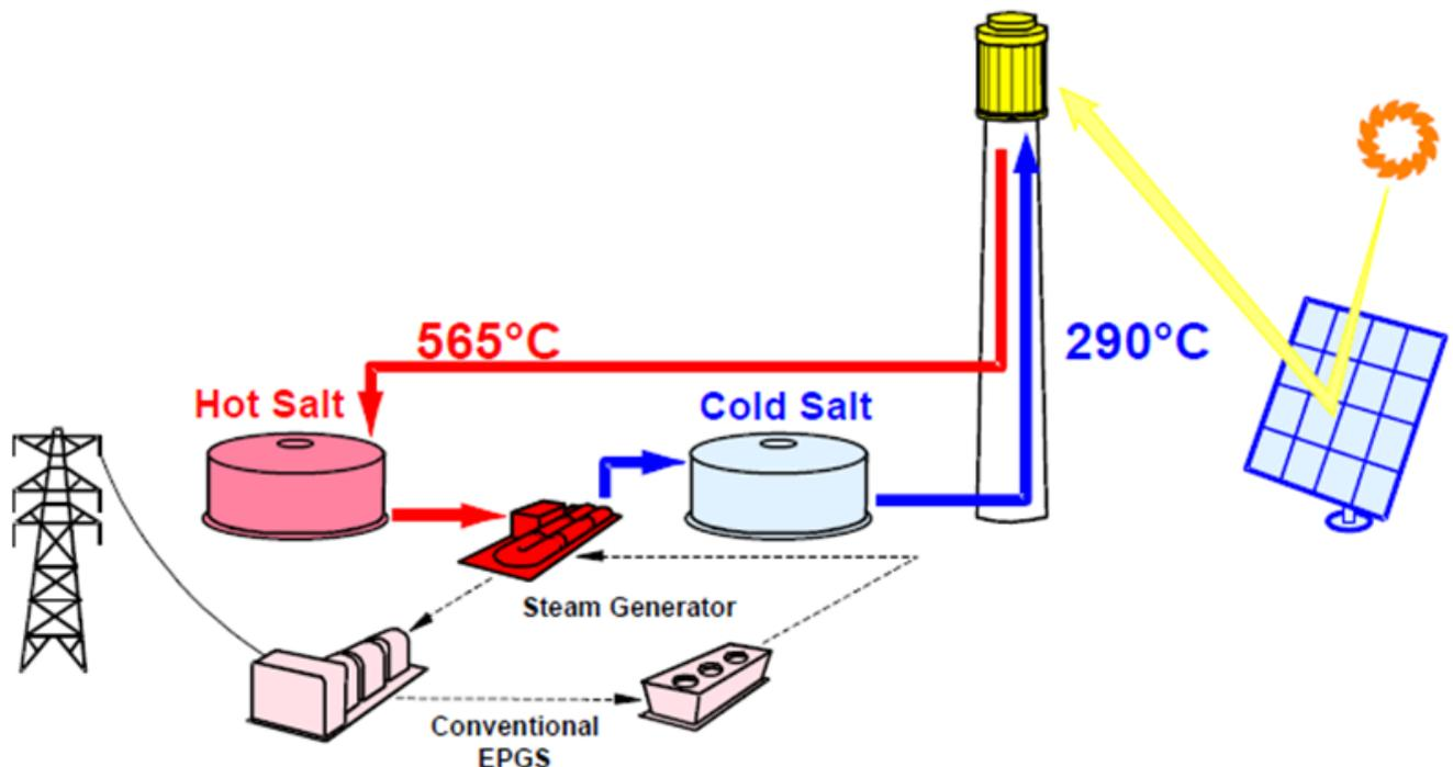
Fig. 4. Schematic of a molten salt power plant [7]
