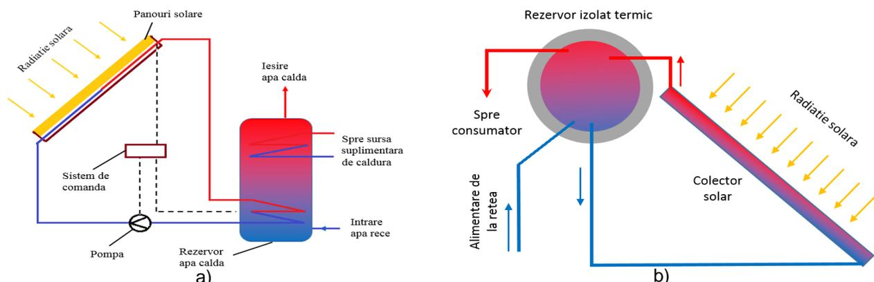
Fig. 3. The structure of a solar water heating system: (a) indirect active system; (B) direct passive system [5]
