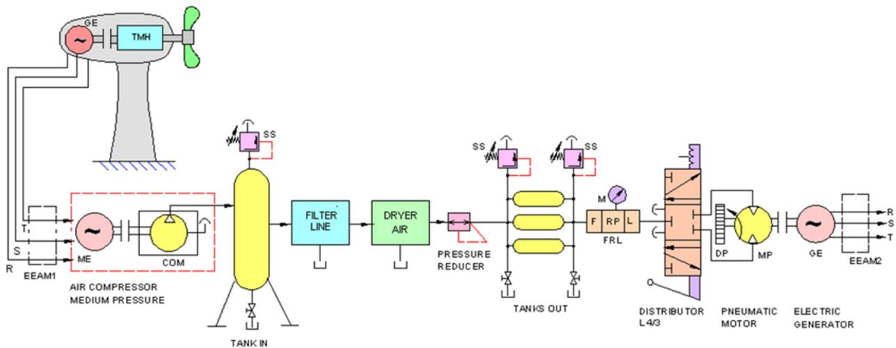
**Fig. 17.** Scheme of a system to capture, conversion and storage of the energy in pneumatic energy
