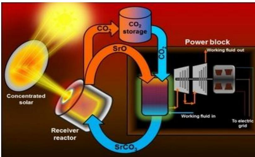
Fig. 5. Electric power plant with thermo-chemical storing system
