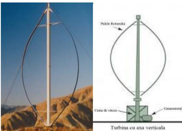
Fig. 9. Vertical axis turbine [5]
