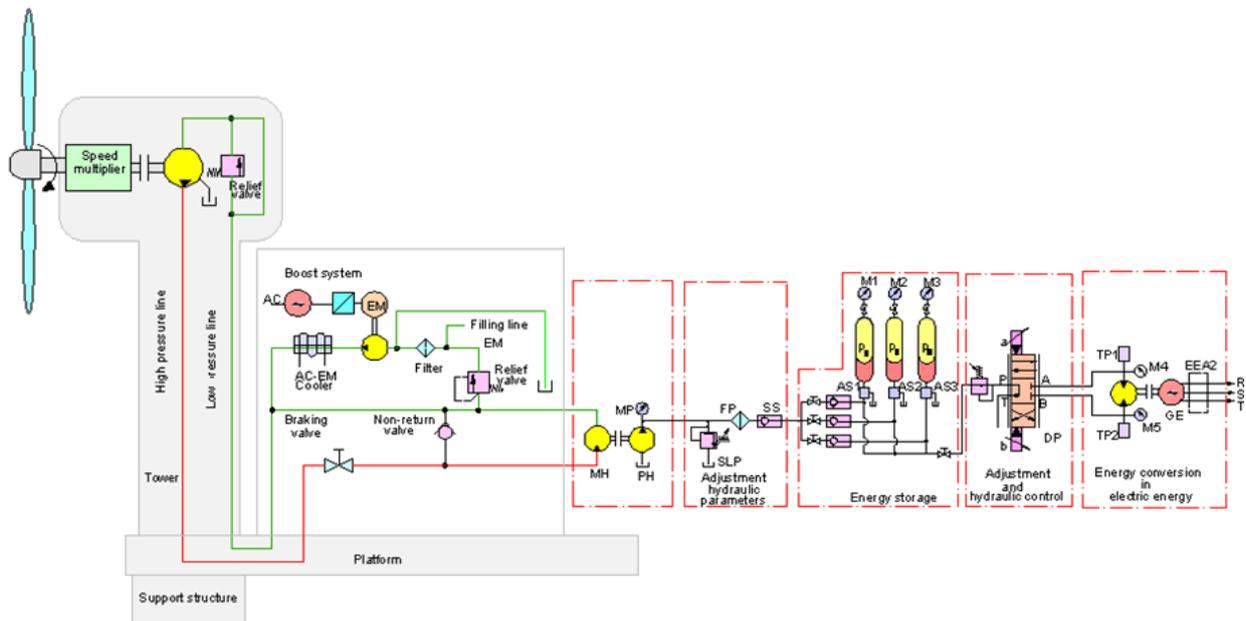
**Fig. 22.** System for Wind energy capture, direct conversion and energy hydrostatic storage
