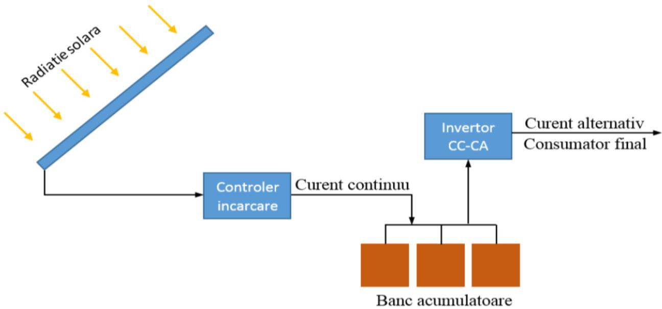
Fig. 8. Simplified diagram of a photovoltaic system [5].
