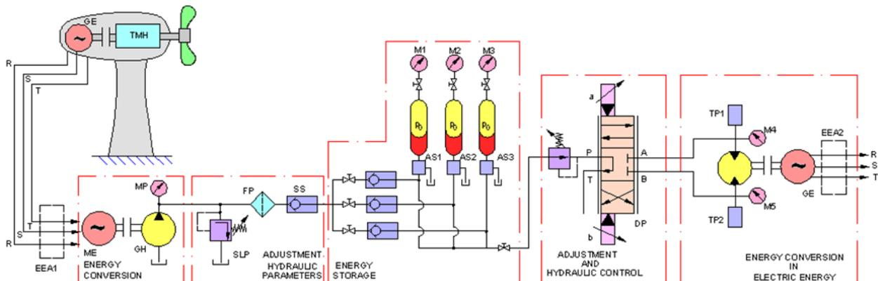
Fig. 21. Scheme of the system for capture, conversion and energy hydrostatic storage
