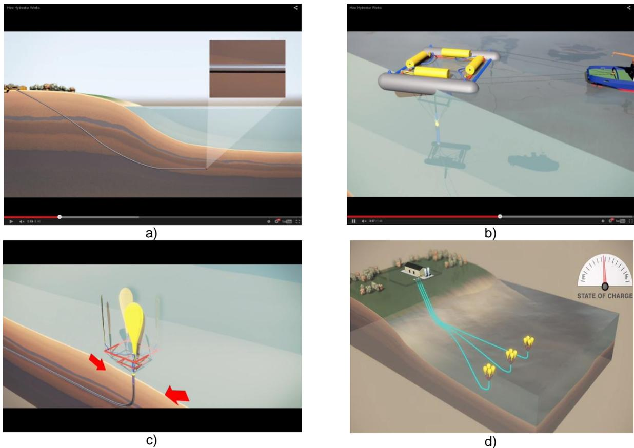
Fig. 14. Pneumatic energy storage technology in deep lakes, [13].
