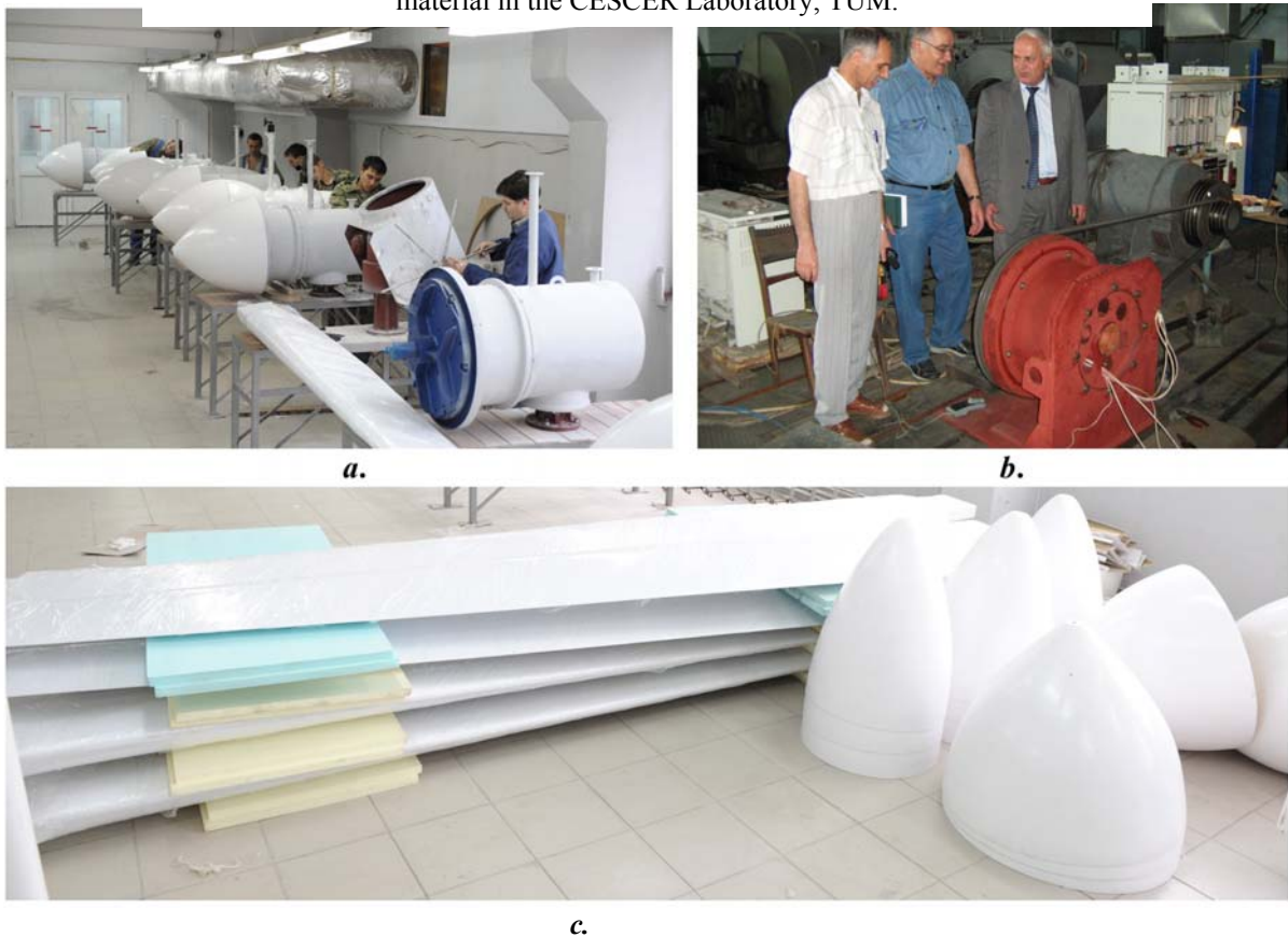
Figure 5: Gondola parts (a) and blades (c) manufactured from composite material in the CESCER Laboratory, TUM; tests of the generator with permanent magnets, Electromas, Tiraspol (b).
