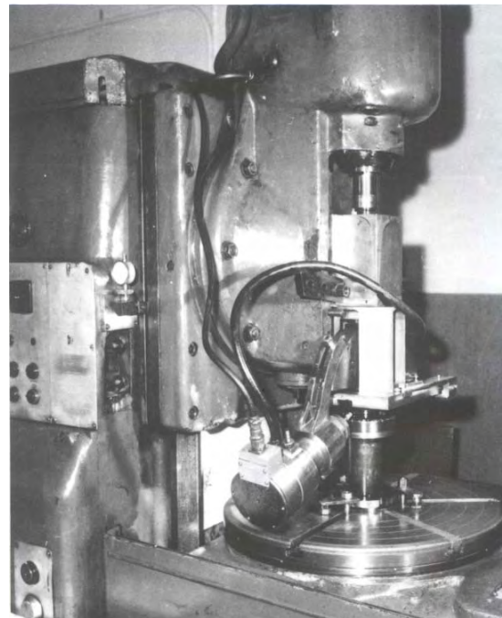
Fig. 4. The device of the realizing for the teeth processing method by rolling using precessional tool.
