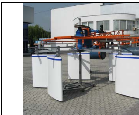
Figure 7: Industrial prototype of micro-hydro power plant for river water kinetic energy conversion
