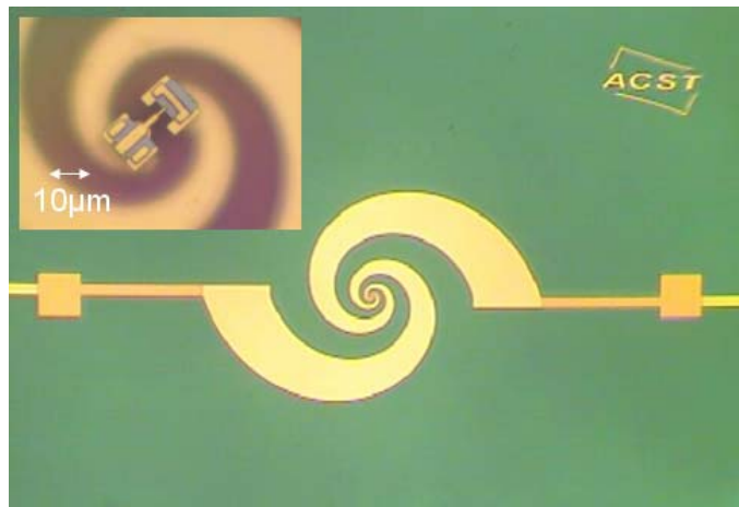
Figure 1: Photograph of the Schottky diode mounted on a spiral antenna. The inset shows the single diode in the center of the antenna.
