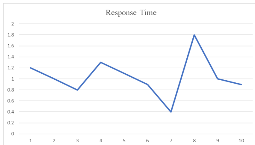
Figure 10. Graph showing the response time of the wheelchair system to movement commands.
