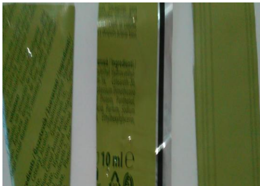
Fig.7. Lacquer with unstable gloss: a. The matte sample exposed to light is glossy; b. Non-lacquered sample; c. Sample which was re-lacquered matte.
