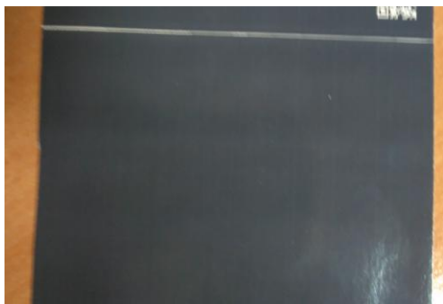
Fig. 3. Printing skips after cleaning the cogwheels.
