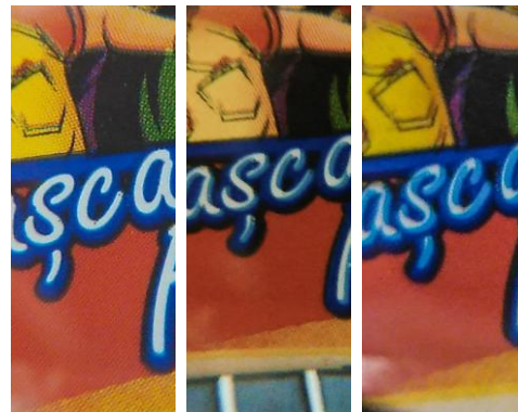
Fig. 8. The Reflex Blue shifted alongside the print length: a. the first repetition; b. the second repetition; c. the third repetition.
