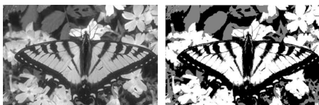
Figure 2. Original image butterfly [20] and segmented image (3 segments).
