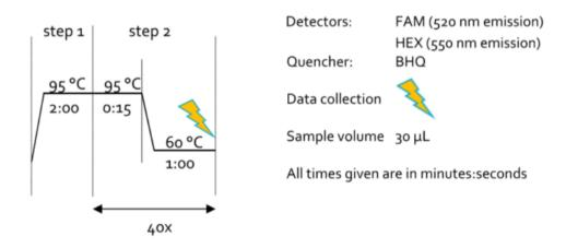
Figure 2. Temperature scheme of thermocycler.
